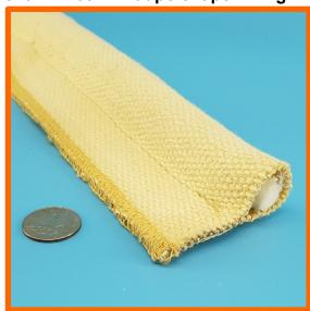
Made from our aramid fabrics and ropes, and metallic mesh ropes, this is a soft and resilient gasket material for effective sealing on light metal flanges and where limited bolting force is available – and where doors and other closures rest on the bulb. The aramid fabric is very abrasion and cut resistant, ideal for high cycle applications. Not suitable for applications involving prolonged sunlight or UV exposure.
